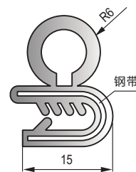
MFT-020 黑色三元乙丙钢带密封条 Black EPDM sealing strip(with steel sheet )
